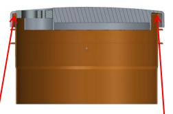
Loose fit gasket holds suction set, but doesn't seal or stay in place creating numerous leak paths
