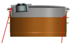
New Gasket is flexible and seals around suction and return line as well as the pail cover. Large over hanging lip provides stability to the gasket. Tapered flange wedges and seals on the inside diameter to create the spill proof design. Works on 5 gallon pails as well as all Graco Hoppers
