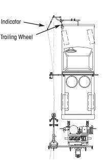
Using the Video Guidance System accessory while restriping a curve, the operator watches the video screen and simply steers the truck to keep the indicator above the line, and the spray guns follow.
