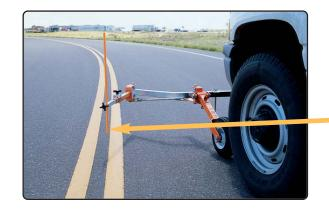
Tracing curves is easy. Simply keep the indicator on the existing line or reference marks. The Line Tracking System compensates for curved lines, indicating where the spray guns will follow.
