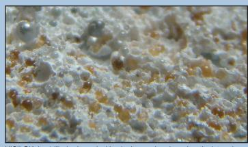
VISILOK durability is shown locking in drop on beads and as the intermix beads are exposed.
